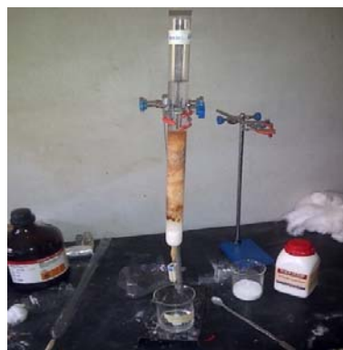
Fig 1: Using the column chromatography to elute the bark and leaf extracts of Erythrina senegalensis and the reagents used.
