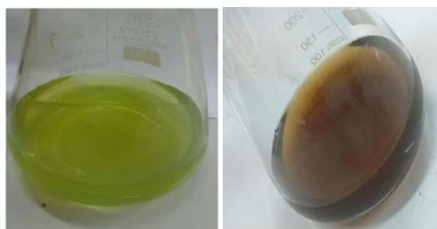
Fig 2: Bioreduction of silver nitrate by Acorus Calamus Leaf extract (a) Aqueous extract (b) colour change after addition of silver nitrate to it.
