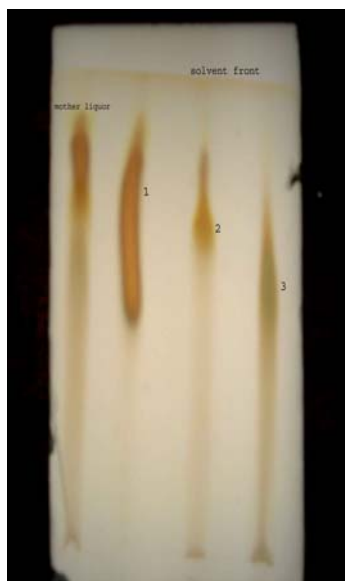
Fig 5: Thin layer chromatographic plate of isolated components from the mother liquor of glycosidic extract.
