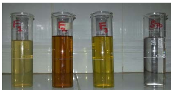
Fig 1: Limit Test for Iron 1., Formulation 1; 2, Formulation 2; 3, Formulation 3; 4, Standard for iron (20ppm)
