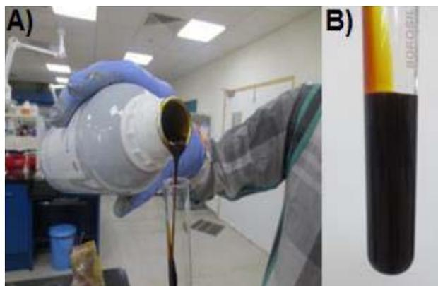
**Fig 1:** Sample extraction procedure for Ginger rhizome: *panel A* - Supercritical fluid extract of Ginger sample, *panel B* – A thick and viscous sample obtained from the SCFE.
