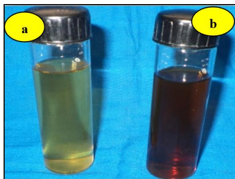
Plate 1: Vials containing the supernatant of T. asperellum in aqueous solution of 1 mM Ag NO 3 at the beginning of the reaction (a) and after 5 days of reaction (b)
