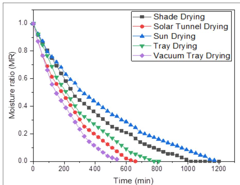
Fig 2: Moisture ratio versus drying time of mulberry leaves in different drying methods.
