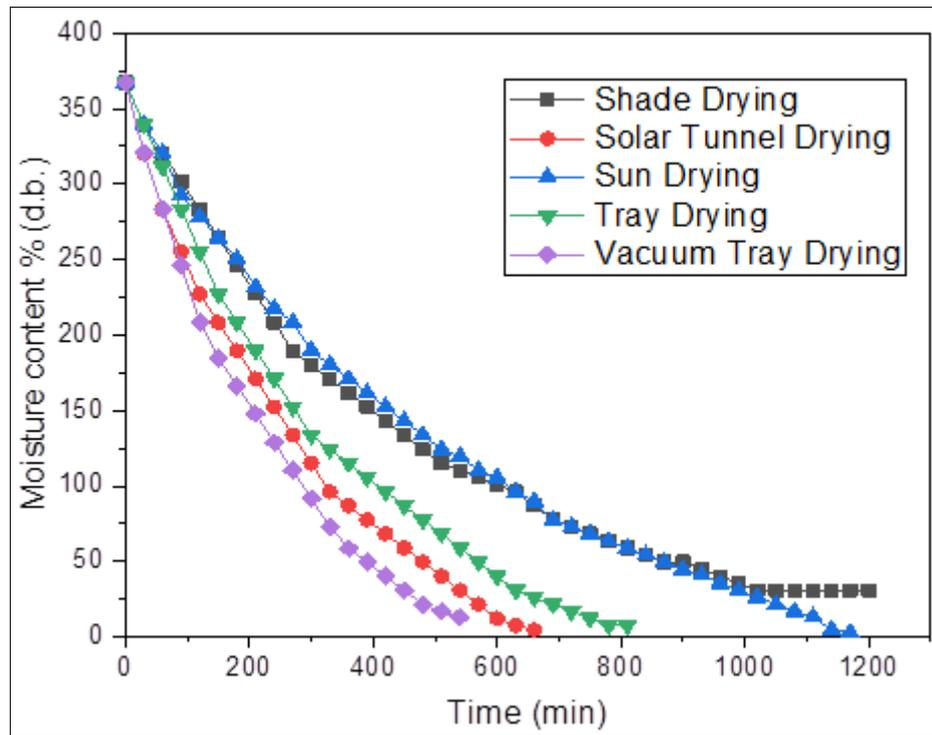
Fig 1: Drying rate curves of mulberry leaves in different drying methods.
