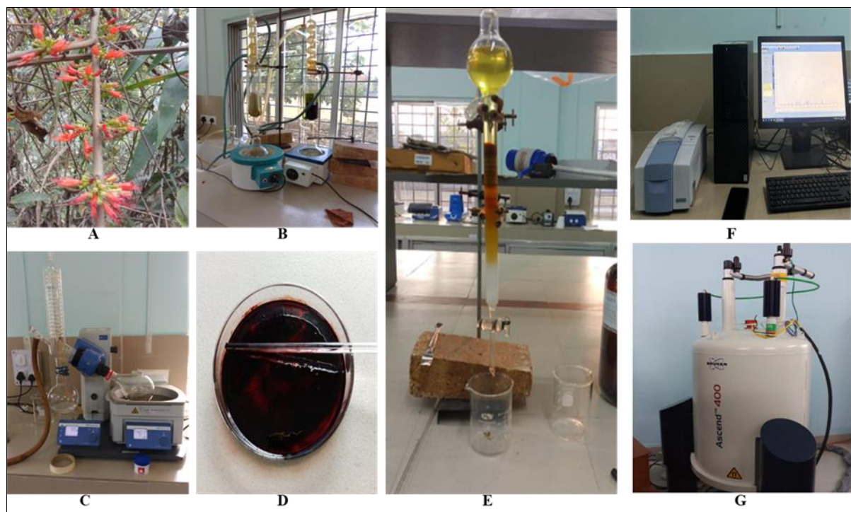
Fig 1: Fresh flower of Woodfordia fruticosa (L.) Kurz (A), Soxhlet Apparatus (B), Rotary Pump Evaporator (C), Dried Extract of WFF (D), Open Silica Column (E), FT-IR Instrument (F), and NMR (G).
